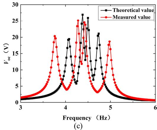
Figure 7. The measured voltage and theoretical voltage at (a) X-direction, (b) Y-direction, (c) Z-direction
