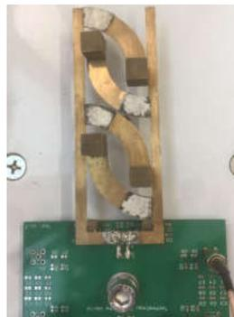
Figure 5. The measured structures of circular arc array piezoelectric VEH.
