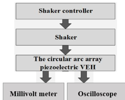
Figure 6. The schematic diagram of measurement.
