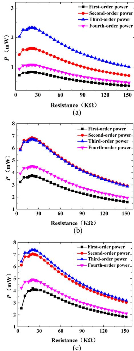
**Figure 8.** Output power of circular arc array piezoelectric VEH at (a) X-direction, (b) Y-direction, (c) Z-direction
