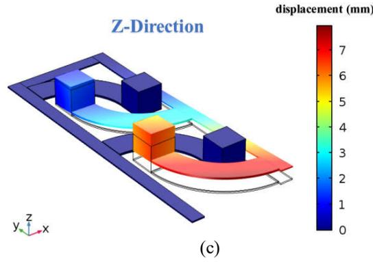
**Figure 3.** The deformation mode of circular arc array piezoelectric VEH (a)X-direction (b)Y-direction (c) Z-direction.
