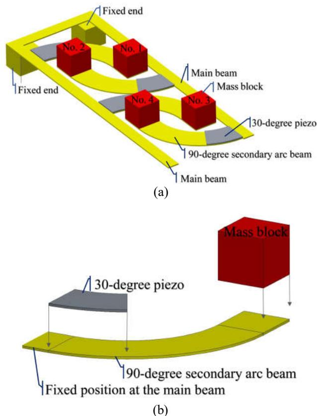
**Figure 1.** (a) The circular arc array piezoelectric VEH, (b) Single circular arc piezoelectric VEH
