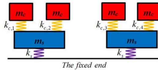
**Figure 4.** The “spring-mass” model of the circular arc array piezoelectric VEH.
