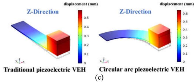
**Figure 2.** The different deformation mode (a) X-direction (b) Y-direction (c) Z-direction.
